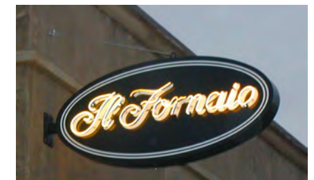
sign panel with exposed neon
